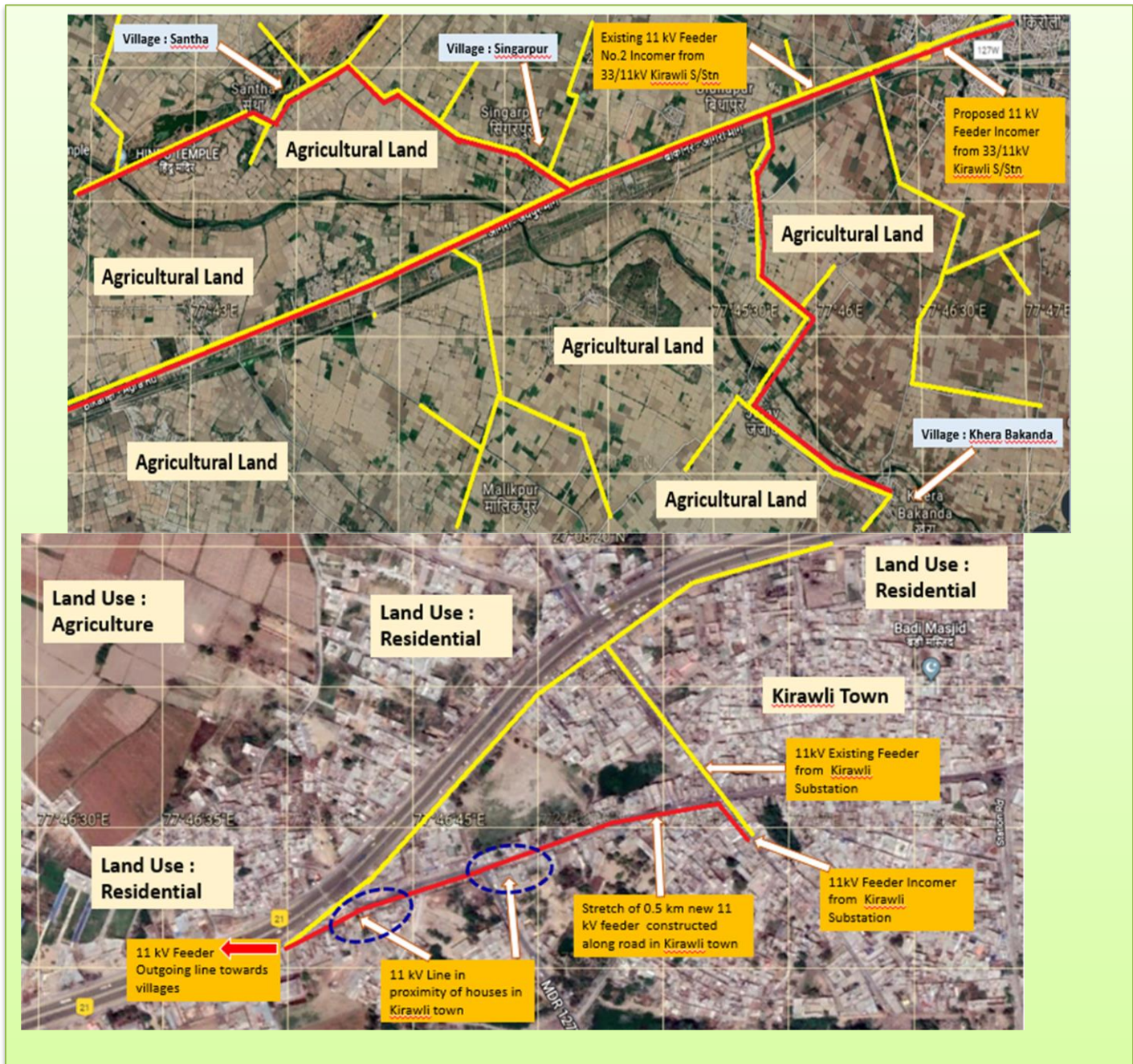
Figure 5: Feeder No 2 (incomer from 33/11 kV Kirawli substation) in PVVNL
